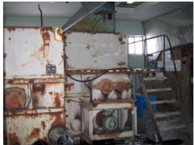
Gusev pasteurizer. Dry substrate enters upper right. Spawned substrate bagged at bottom left.
